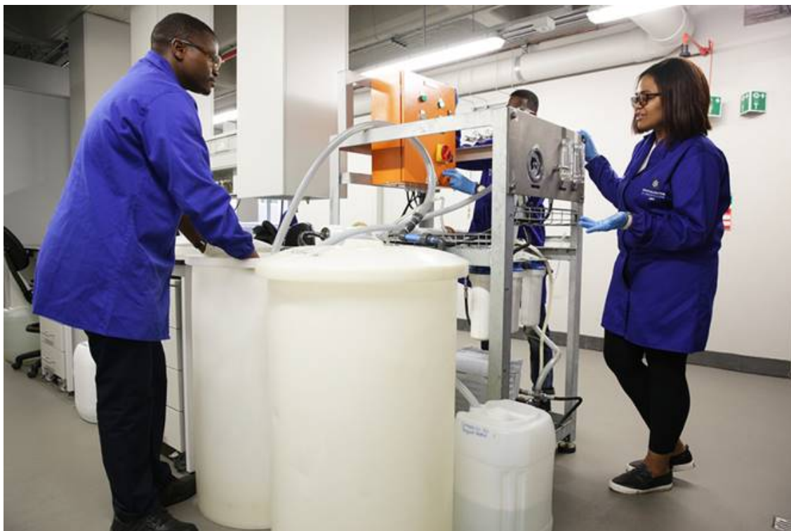
Caption: UCT Chemical engineering students work with the reverse osmosis plant to desalinate seawater. Credit: Robyn Walker/UCT
