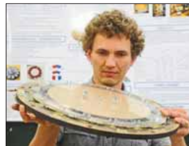
Round and round: Hartmut Jagau with the generator that he designed using magnets from discarded hard drives.
