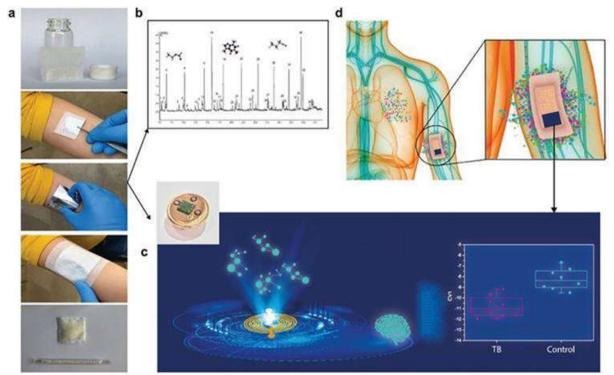
Study schematics: a) Skin headspace sampling procedure. The samples are transferred into glass tubes for two analyses: b) Gas chromatography–mass spectrometry analysis of the collected samples; and c) nanomaterial-based sensor array applied to a machine learning analysis. d) A wearable device applied directly on the skin.
